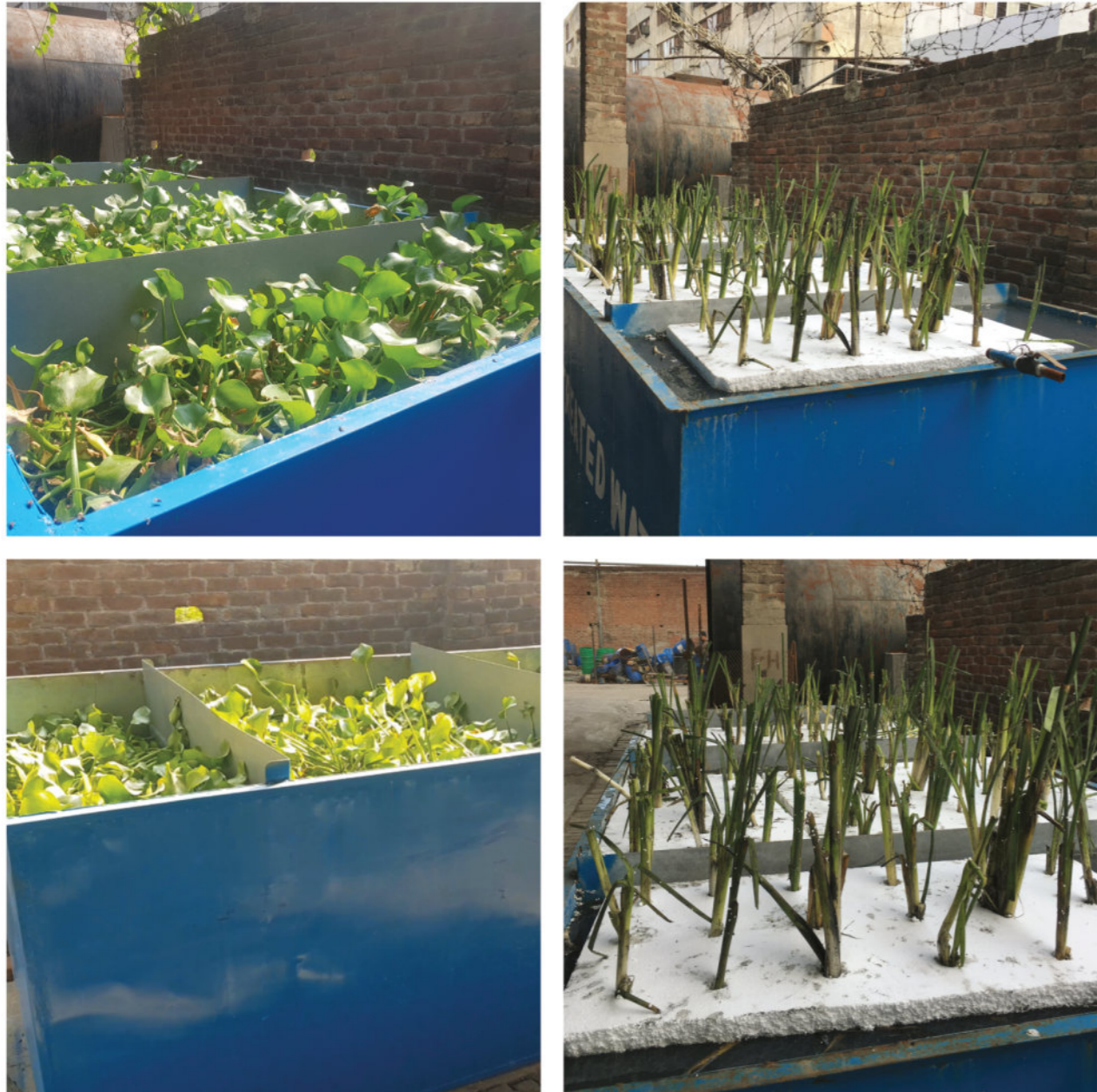
Plate 1: Bio-remediation pilot for chrome tanning wastewater
